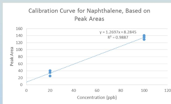
Figure 2- Calibration curve for naphthalene extracted from aqueous solutions using a 100 μm SPME fiber; similar curves were created for each PAH.
