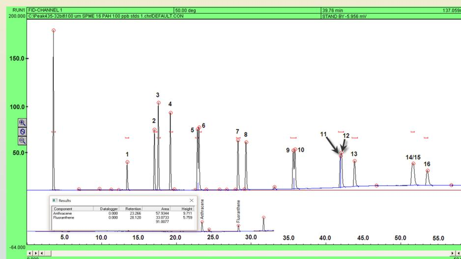
Figure 1- Chromatogram from 100 ppb solution of all 16 PAHs using a 100 μm SPME; inlay shows the results from a river water sample that showed the method was able to successfully detect PAHs in environmental samples using the 30 μm SPME fiber.
